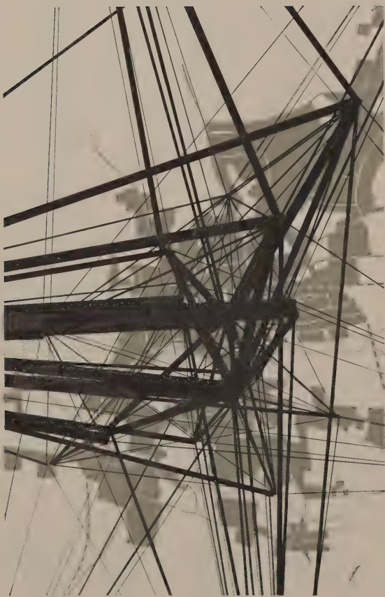
48 A desire line diagram (see para. 84) for work journeys in a small town.
